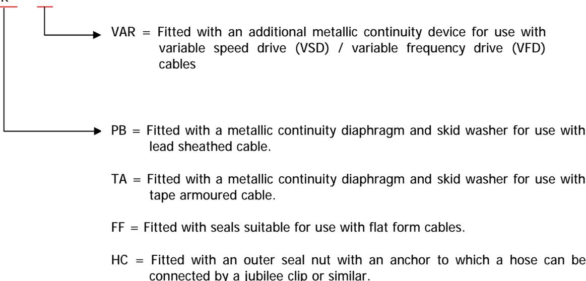
The gland and seal sizes are determined by the entry thread and cable range take sizes:
